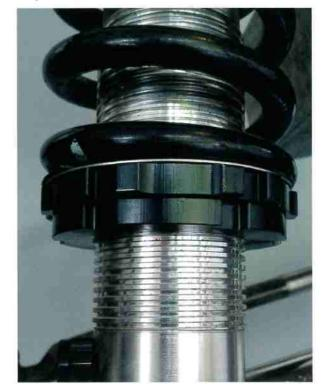
The suspension heights are listed as 335mm front and 325mm rear, with a tolerance of 5 percent, meaning the rear suspension can be between 309mm and 341mm. Rear height of 310mm is within the acceptable range.
